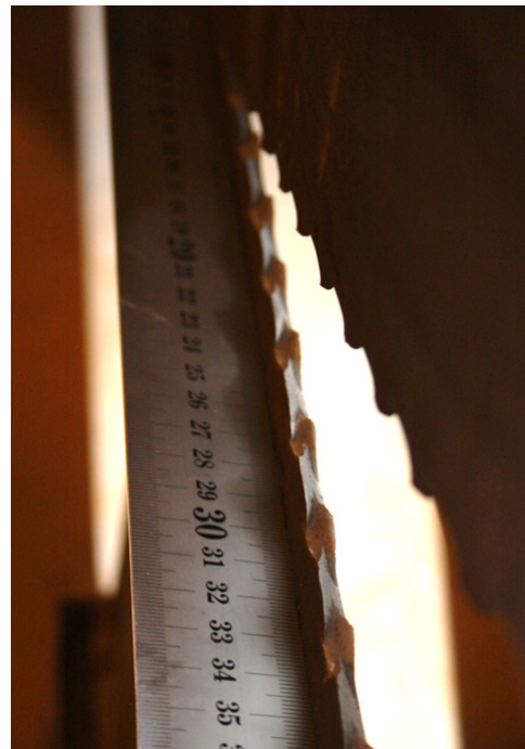
Figure 1: Repeated crack tip flipping in large scale testing of a normal strength steel plate subject to mode I loading.
